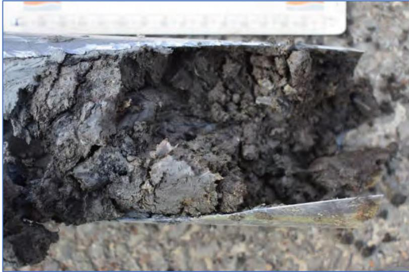
**Plate 4: TP26 peat at base of core at 5m below ground level**
