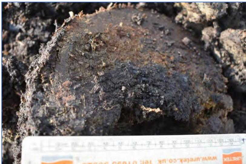
**Plate 5: MW0 Fibrous peat at base of core at 1m below ground level**
