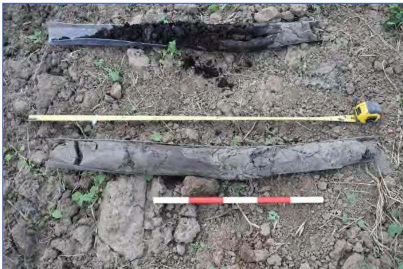
**Plate 8: WS14 organic silts and clays at 2-3m (top) overlying sterile stiff clay and sand at 3-4m (bottom)**
